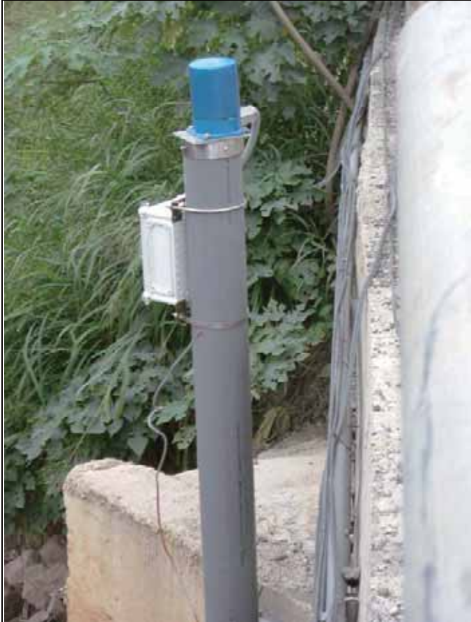
TW-265S with Wireless Transmitter, Battery or Solar powered. License free RF module ranged at 150~500m.
