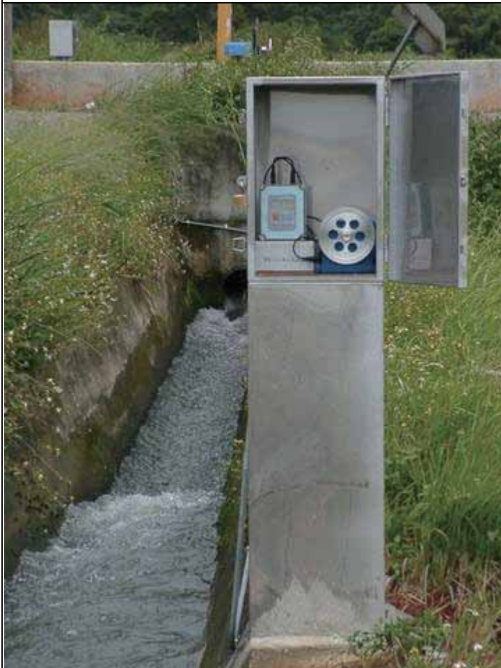
TW-252S connected with FSK transmitter to control room.
